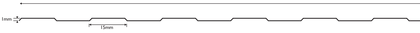
Our Petrochem ZX ® profile increases strength with no loss of overall coverage - 66 stiffening ribs per metre
